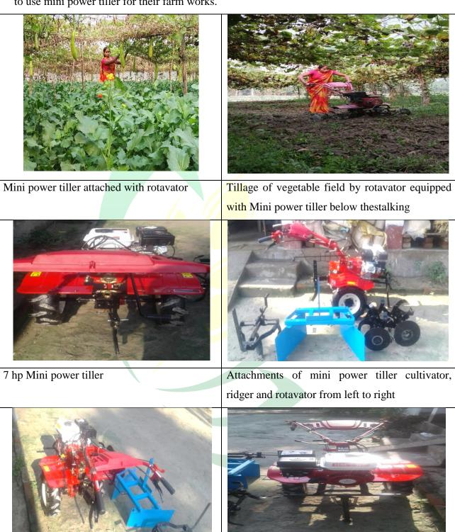
Fig.2: Mini power tiller different attachments with rear and front view
